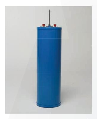
The Mavitek MVK series Bandpass Cavity filters in 6" (152mm) diameter are designed and produced to meet the high selectivity. The MVK series filter are blue enamel painted copper. The connectors are silver-plated and PTFE insulated. With high "Q" values they achieve maximum isolation and superior performance with 500kHz Rx/Tx frequency shift.
